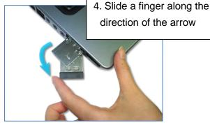
5. Rotate the panel for a right angle
